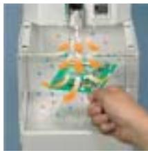
**Different pulsed air emissions can be selected by the solenoid valve**
